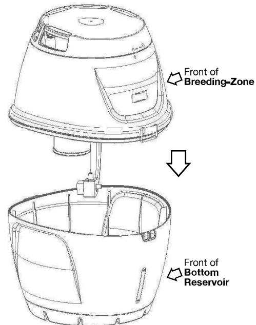
**Step 9:** Attach the Breeding-Zone to the Bottom Reservoir. Align the latches at each side of the Mosquito Preventer, then lock each of the latches.
