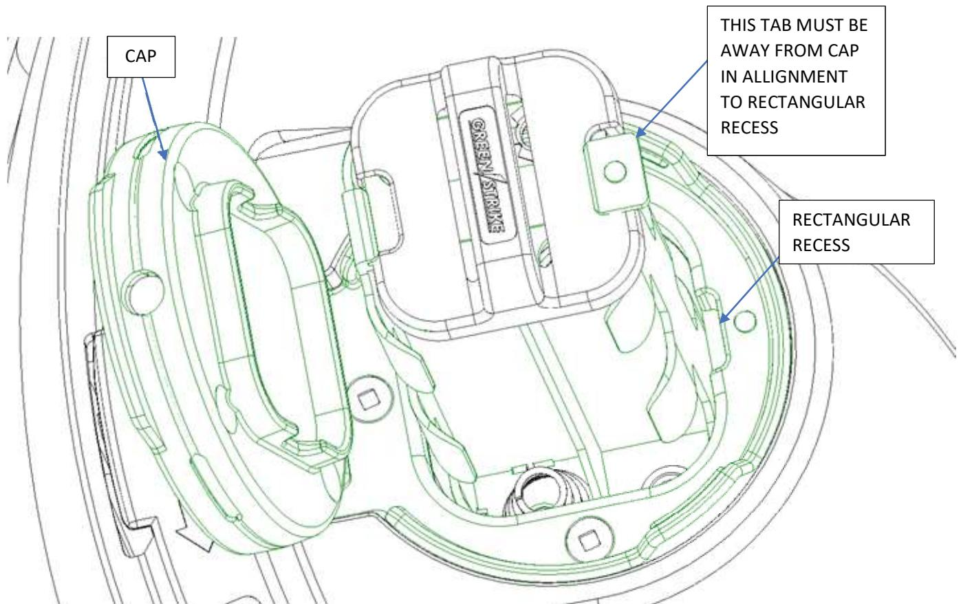
If the above diagram is followed while inserting the **Battery Tray** after changing the Batteries or during SET UP, then the **Battery Tray** will never get stuck
