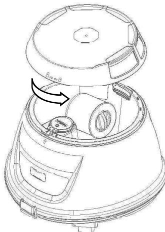
**Step 3:** Rotate the lid of the **Breeding-Zone** to unlock and remove the lid. This will give you access to the **Reactor**, **Batteries**, **Remote** and **Landing Strips**.
