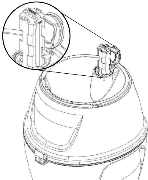
**Step 5:** Open the battery compartment and retrieve the battery tray. Insert the 8 AA batteries into the tray. Return the tray to the battery compartment with the little black square facing the **Landing Strips**. Close the cover firmly by hand.
