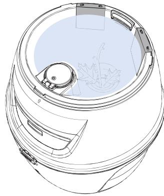
If the **Breeding-Zone** water level has dropped, simply press the **add water** button
