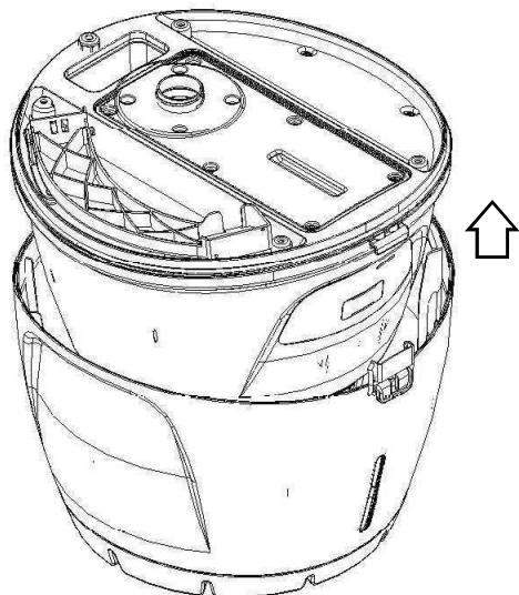
**Step 2:** Separate the Breeding-Zone from the Bottom Reservoir.
