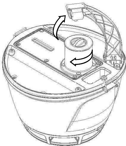
**Step 8:** Attach the **Reactor** to the **Breeding-Zone** and rotate until the **Reactor** is locked in place. Raise the pump control arm until it clicks firmly into a locked position.
