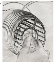
Remove the lamp by using your thumb and forefinger and pulling the lamp towards you.
